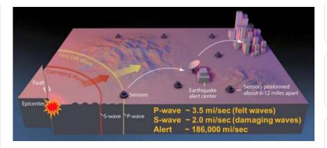
Primary (P) wave energy, which rarely causes damage. Using P-wave information, we first estimate the location and the magnitude of the earthquake. Then, the anticipated ground shaking across the region to be affected is estimated and a warning is provided to local populations. The method can provide warning before the Secondary (S)-wave arrives, bringing the strong shaking that usually causes most of the damage.
